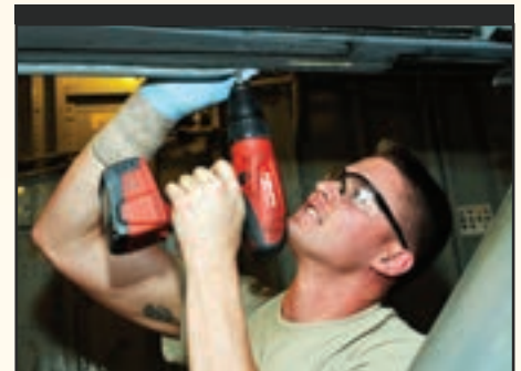
U.S. Air Force crew chief, Airman 1st Class Trevor Foisy, removes a gasket from the wheel well of a KC-135 aircraft at the Utah Air National Guard Base in Salt Lake City April 14, 2012.
