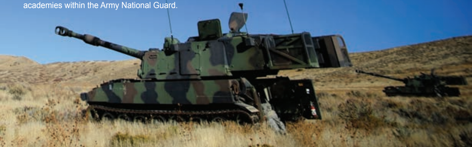
Members of the 640th RTI conduct live-fire training on a M109A6 Paladin self-propelled howitzer. Soldiers load the big guns.
